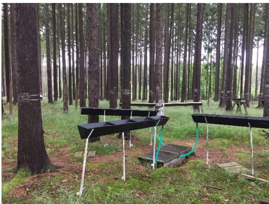
Fig. 7 The plastic gutters for capturing precipitation water under the stand
